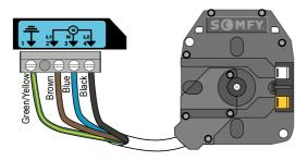
Connect the motor wires into terminals 1, 2, 3 and 4 as illustrated above.
