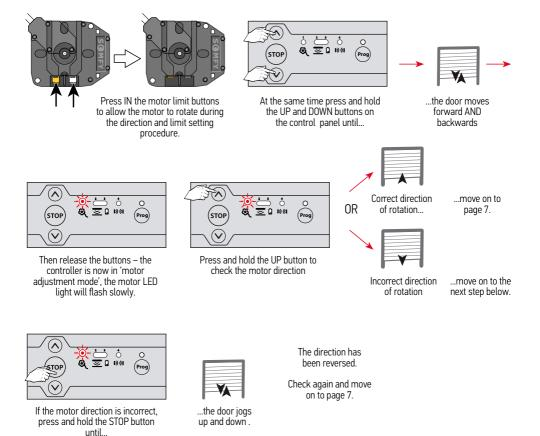
In motor adjustment mode, the Up & Down control buttons are in 'hold to run' mode - you must press and hold the button in to operate the door up and down.
