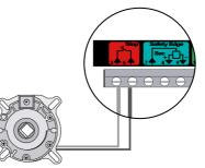
Connect the electrical safety brake into terminals 5 and 6.
